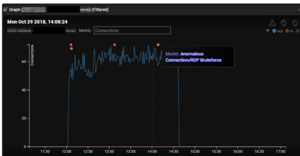
Figure 21: A clear plateau in increased internal connections can be seen. Every colored dot on top represents an RDP brute force detection
